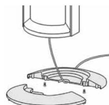
First assemble the two halves of the pedestal. Then pass the power cord through the hole in the center and mount the pedestal to the fan. Make sure that you lead the cable through the cable entry.
